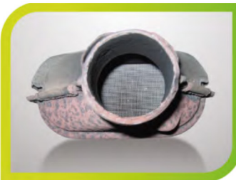
Clogged CATALYTIC CONVERTER
